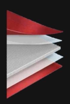
Honeycomb Panel consists of two high-modulus and high strength face sheets are adhesively bonded to Abstract Quarter Honeycomb. The result is a high-strength, lightweight structure that behaves much like an I-Beam.
